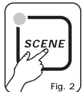
The speed of change between the scenes can be controlled by **RATE ▲** and **RATE ▼** (see par. 5.1).
